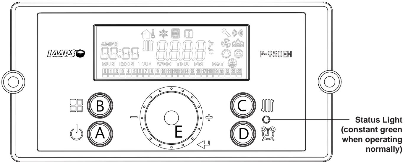
The **Control Display** has a Control Dial (E), 4 buttons (A, B, C, D), and a Liquid Crystal Display (with 72 back-lit segments). This section of this manual gives instruction on how to navigate into the many functions of the Mascot FT and to change temperature set points, set system variables and controller parameters.
