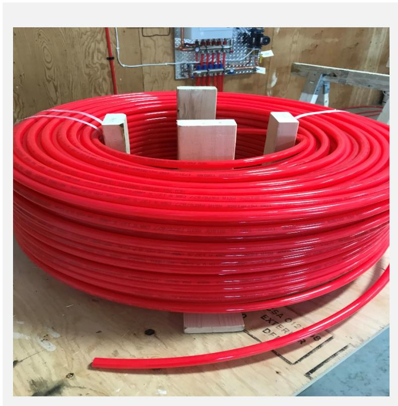
10- After placing the roll of tubing on the hub, screw the section you had set aside onto the uncoiler, so that it holds the roll of tubing in place.
